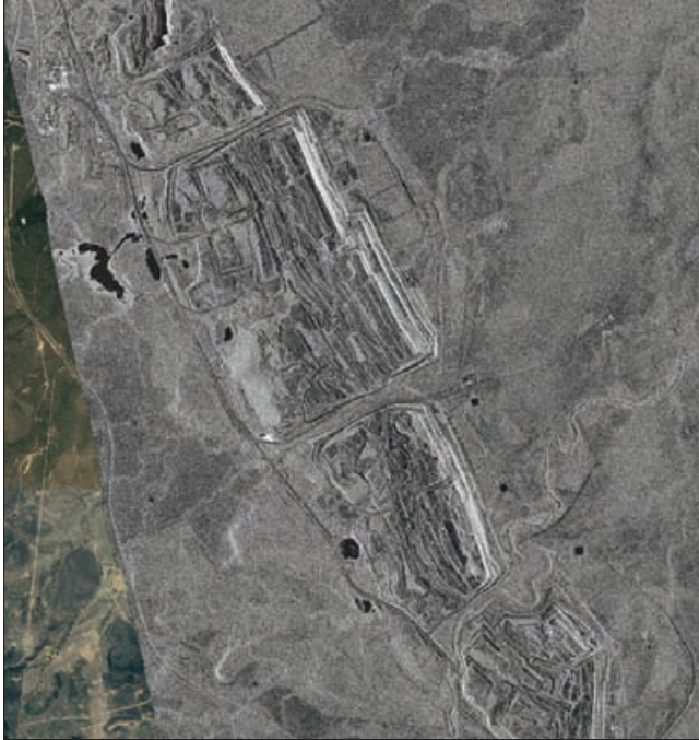
Optical and SAR can detect changes in stockpiles. Source: Terra-SARX. 2018/08/04. Resolution: 3m ●●●
