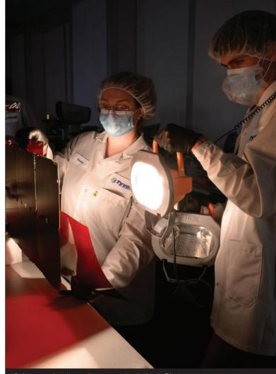
Solar panel string voltage test (red glow). Photo courtesy NASA ●●●
