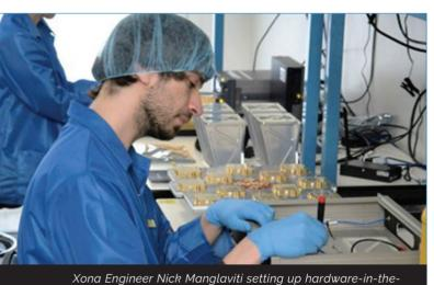
loop testing at Xona's R&D lab in San Mateo, California. (Photo: Xona Space Systems) ●●●
