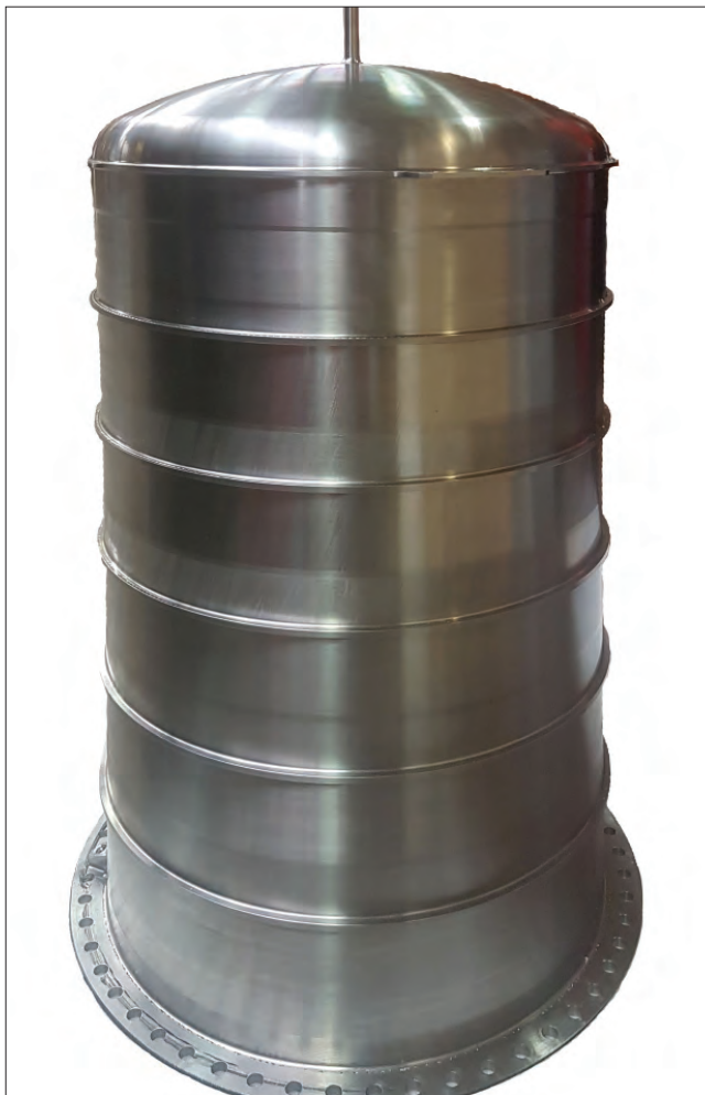
First WAAM full-scale prototype of a titanium pressure vessel to be used in future manned missions for space exploration ●●●
