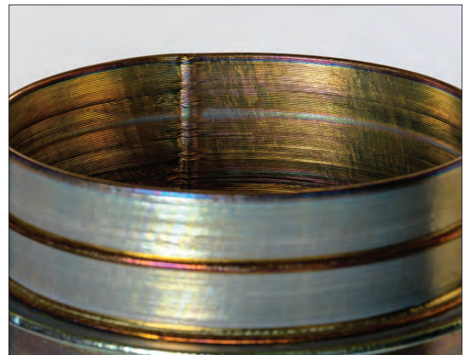
First WAAM full-scale prototype of a titanium pressure vessel to be used in future manned missions for space exploration ●●●
