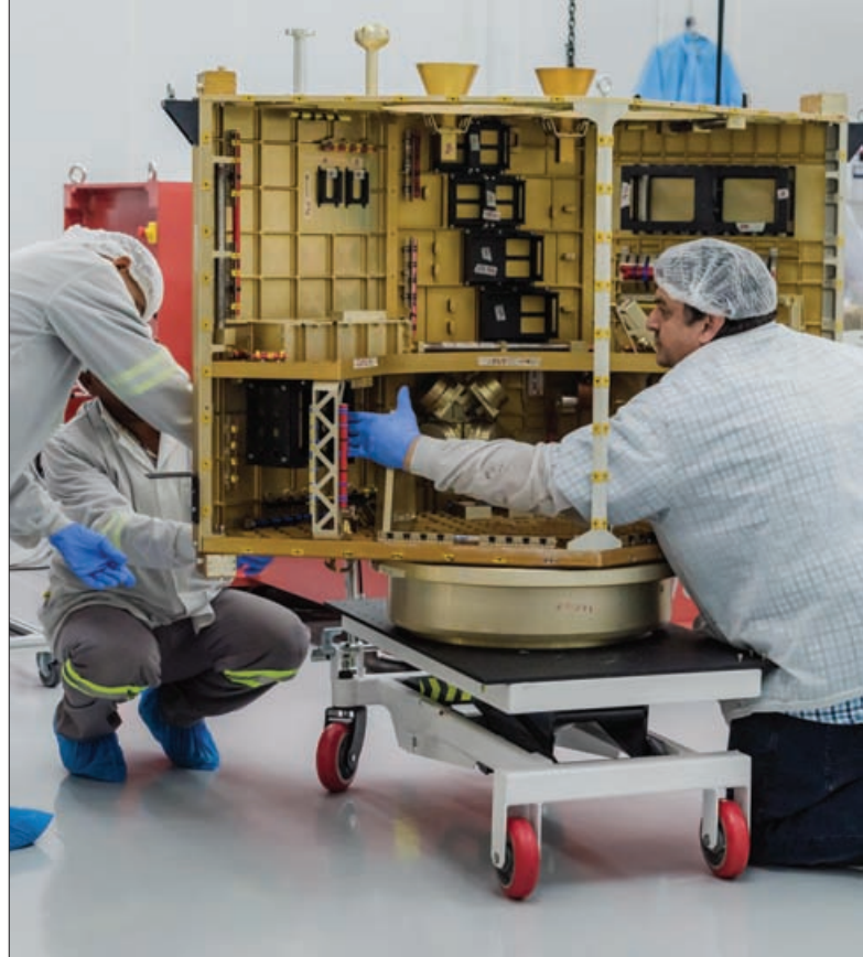
Engineers performing assembly tasks on the EOS SAT-1 at Dragonfly Aerospace facilities. Photo courtesy Dragonfly Aerospace ●●●
