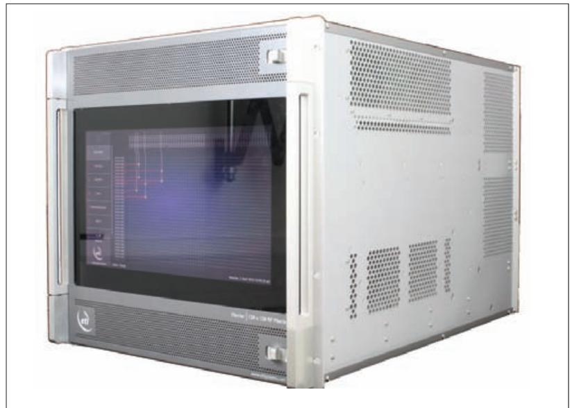
ETL Harrier 128x128 RF Switch Matrix. Photo courtesy ETL Systems ● ● ●
