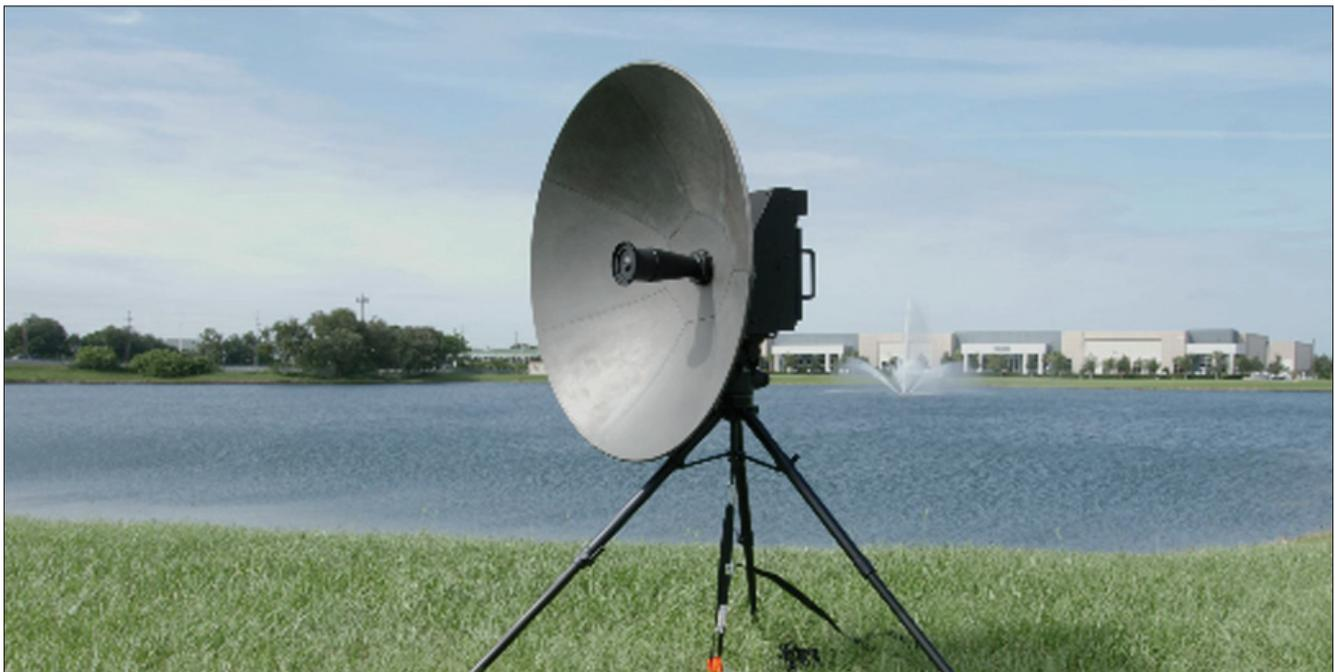
Mobile by design, and the smallest of Comtech's Family of Troposcatter Systems, Comtech's Compact Over-the-Horizon Transportable Terminal (COMET™) is the world's smallest and lightest modular, man-packable troposcatter system. COMET was developed to provide resilient communications in contested environments addressing a wide range of tactical mission needs. Photo courtesy Comtech ●●●
