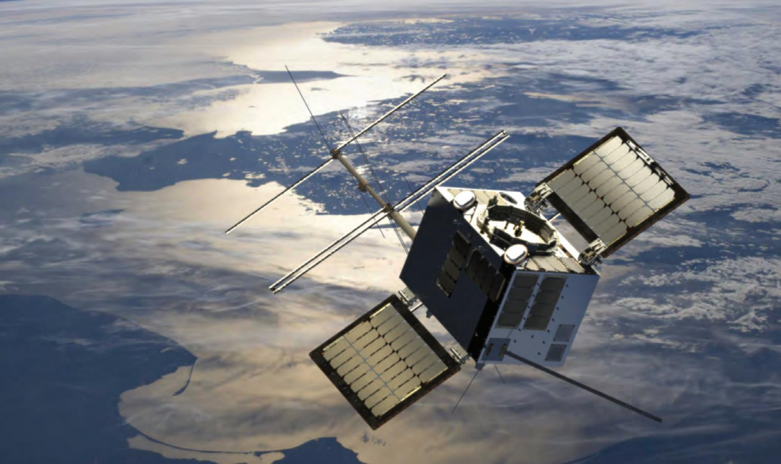
In addition to an AIS receiver and VDES two-way communication device with Yagi antenna, NorSat-TD carries four experimental payloads ●●●
